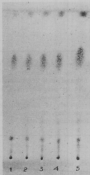
Figure 1. Tlc separation of pulp oil extracts from ripening mango pulp (variety Alphonso) on silica gel plate. See Experimental Section for tlc details. 1, raw. 2, half ripe. 3, table ripe. 4, fully ripe. 5, over ripe.
